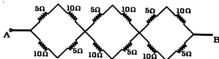
Determine the effective resistance of the given circuit between points A and B.
