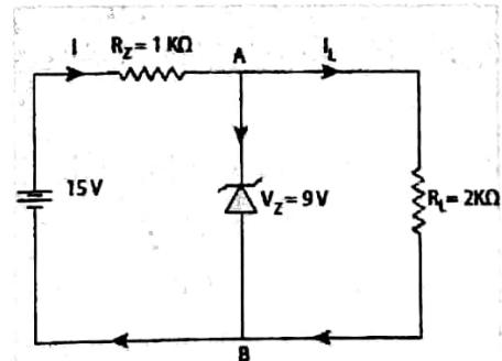
Find the current through the Zener diode when the load resistance is 1kΩ. Use diode approximation.
