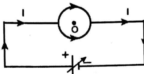
Magnetic induction at the centre of the ring as shown in diagram.
