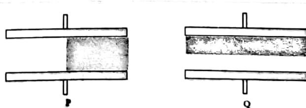
Capacitors P and Q have identical cross sectional areas A and separation d. The space between the capacitors is filled with a dielectric of dielectric constant  $\epsilon_r$  as shown in the figure. Calculate the capacitance of capacitors P and Q.
